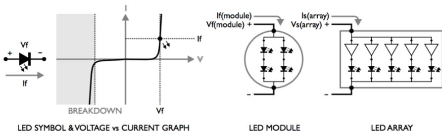
So before you can select the correct LED driver you must determine the fixture type and then gather the drive characteristics from the manufacturer:
